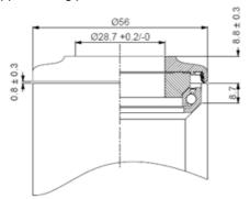
In case of assembling on DCR frameset, cables will enter close to the levers and will go out under the stem, passing across the spacers, top cover of 56 mm (10) and compression ring (11).
