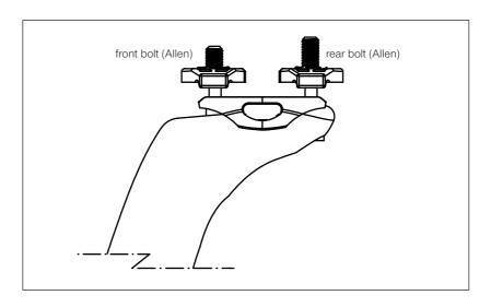
For type B seat posts (equipped with front bolt with adjusting wheel and rear socket head bolt) follow the fitting plan below:
